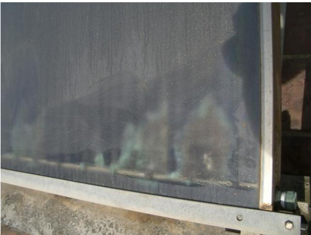
Fig. 6: Corrosion due to Salty Air
