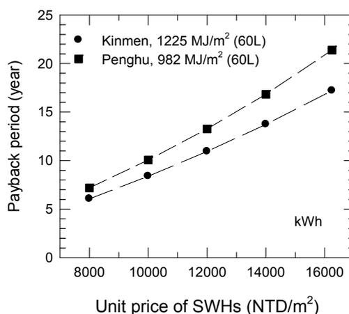
**Figure 7.** Payback period as a function of  $L/A_{sc}$ ,  $IC_o = 12,250$  NTD/m<sup>2</sup>.
